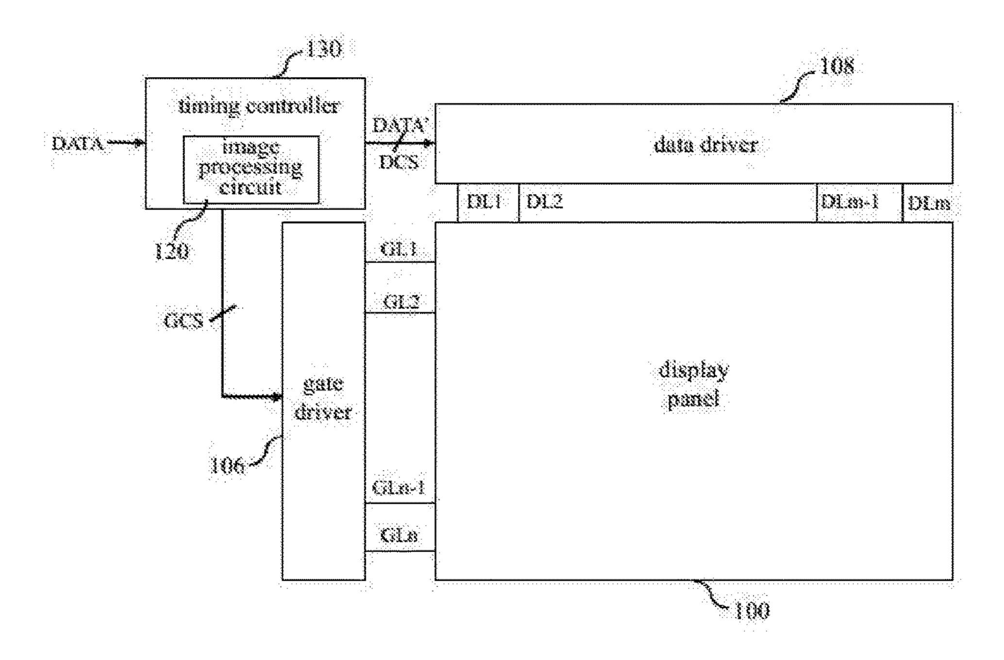
IMAGE PROCESSING CIRCUIT AND DISPLAY DEVICE USING THE HISTOGRAM ANALYZER TO PERFORM A DIFFERENTIAL SHIFT AND EXTENSION SHIFT OF IMAGE DATA GRAY LEVEL TO ADJUST GRAY LEVEL RESPECT TO THE BRIGHTNESS IMAGE LEVEL
