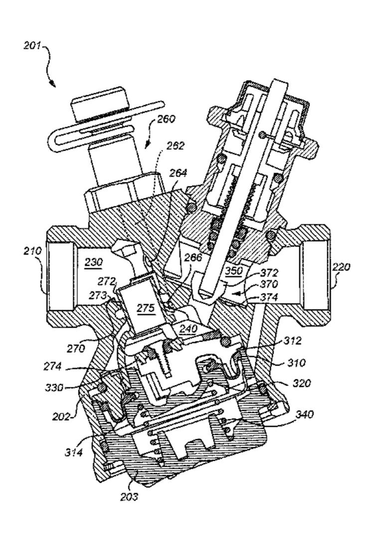
closing arrangement in its open positions is configured to allow for fluid communication between the first chamber and the second chamber via the closing arrangement.
