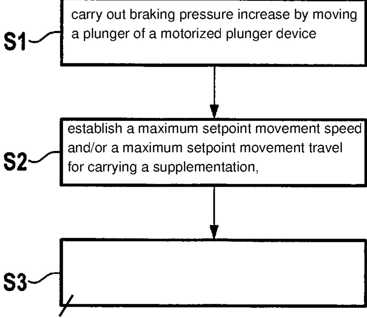
activate a motor of the motorized plunger device while carrying out a volume supplementation, so that the maximum actual movement speed corresponds to the maximum setpoint movement speed and/or the maximum actual movement travel corresponds to the maximum setpoint movement travel
