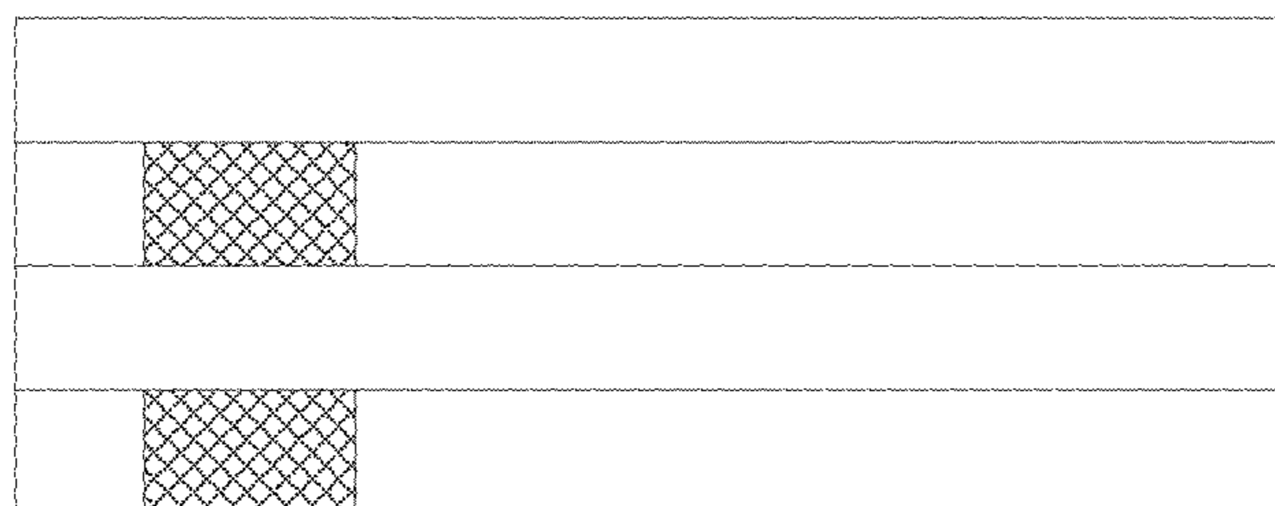
(c) 2-symbol short PUCCH can be transmitted in any two symbols within the configured PUCCH symbols
