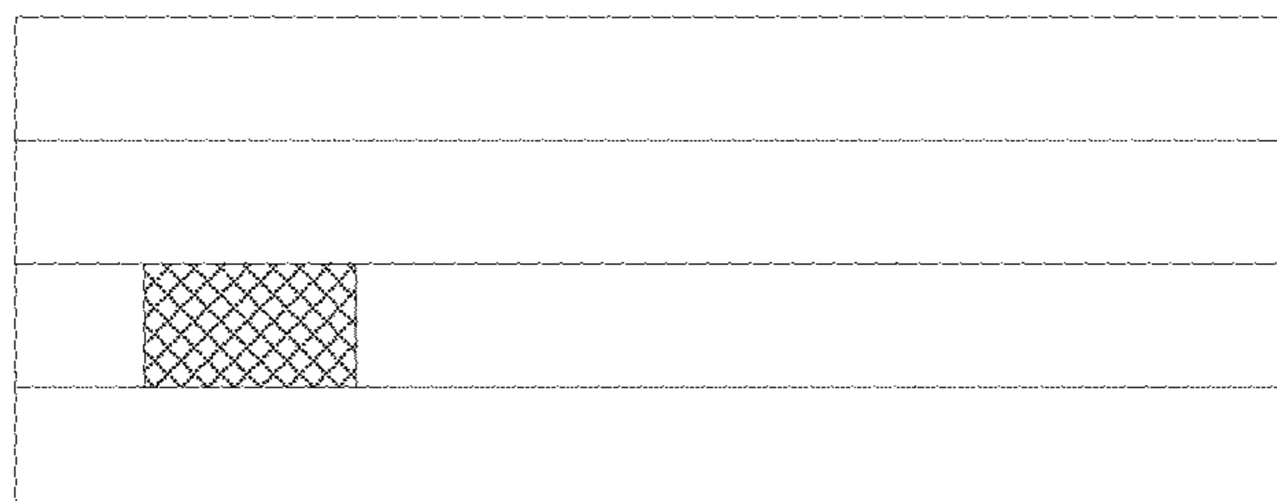
(a) 1-symbol short PUCCH can be transmitted in any one of the configured PUCCH symbols
