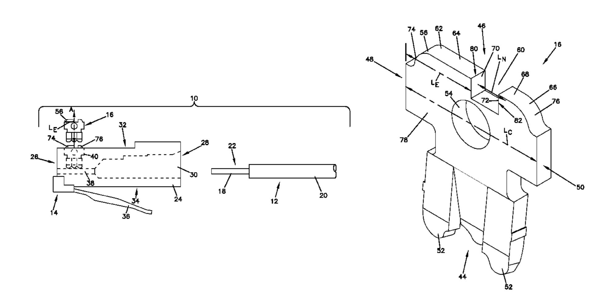
first push surface that is generally at the same height as a second push surface defined by an uppermost portion of the second engagement surface. The notch is defined by a front vertical wall spaced from a rear vertical wall, wherein the front vertical wall is positioned at a distance of at least half the length of the contact from the front end of the contact.
