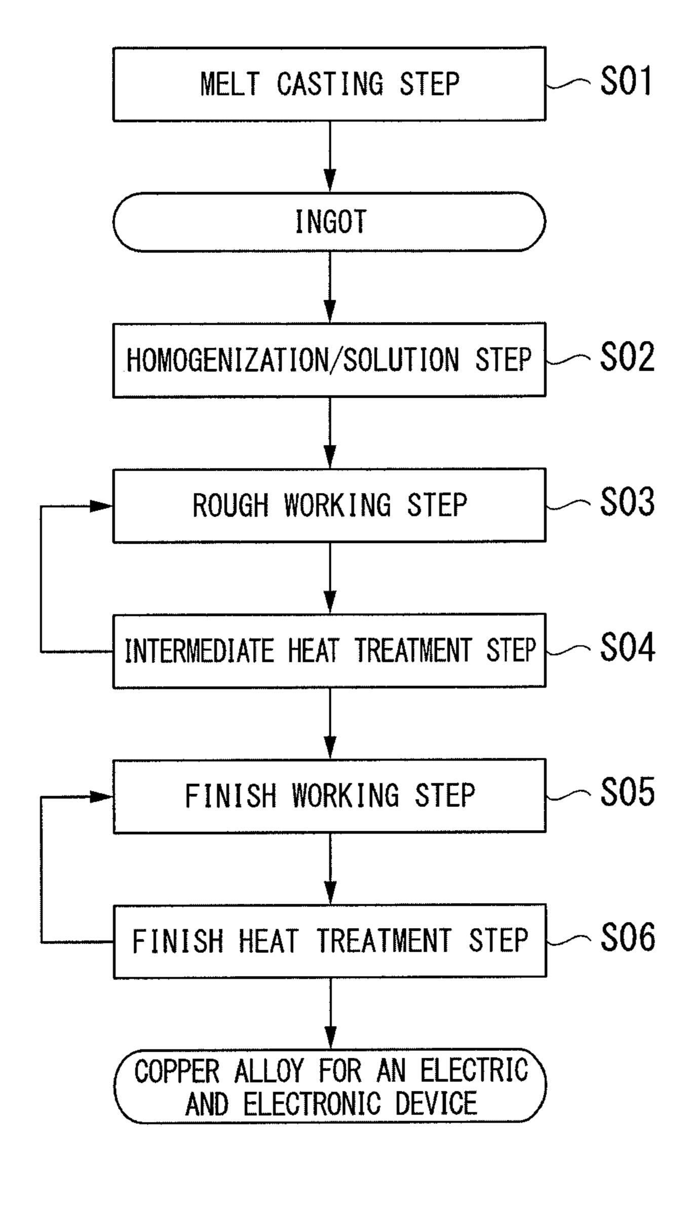
**COPPER ALLOY FOR** ELECTRONIC/ELECTRICAL DEVICE, COPPER ALLOY PLASTICALLY-WORKED MATERIAL FOR ELECTRONIC/ELECTRICAL DEVICE, **COMPONENT FOR** ELECTRONIC/ELECTRICAL DEVICE, TERMINAL, AND BUSBAR
