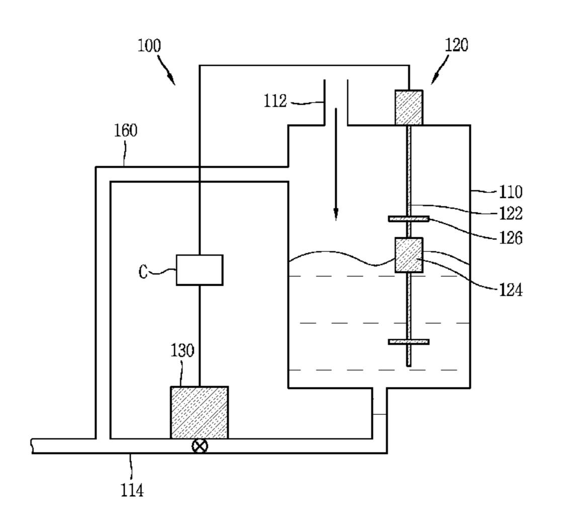
a control unit configured to calculate a micro flow rate of the fluid collected in the container using information acquired from at least one of the fluid level gauge and the control valve.
