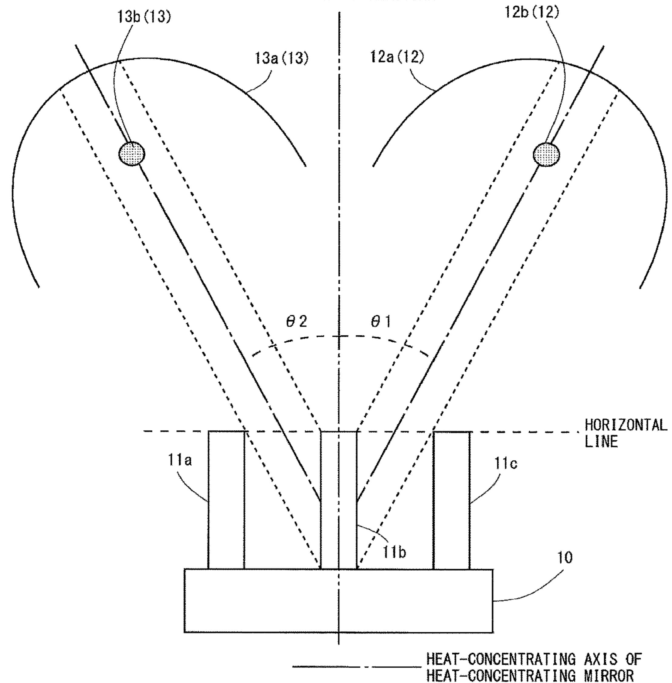
Fig. 2 14 INSPECTION APPARATUS 15 TEMPERATURE INFORMATION TL. TEMPERATURE INFORMATION TL ARITHMETIC OUTPUT FROM THERMISTOR 13b OUTPUT FROM THERMISTOR 12b UNIT 12b (12) 13b (13) 12a (12) 13a (13) HEAT-CONCENTRATING AXIS OF
