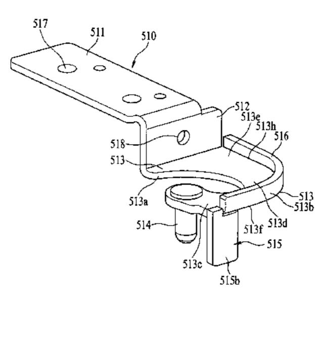
of the second door, a hinge bracket coupled to the second door, and an indented member provided between the hinge shaft and the hinge bracket, the indented member being moved through the hinge hole so as to allow the entire second door to escape from the door frame when the second door is opened.
