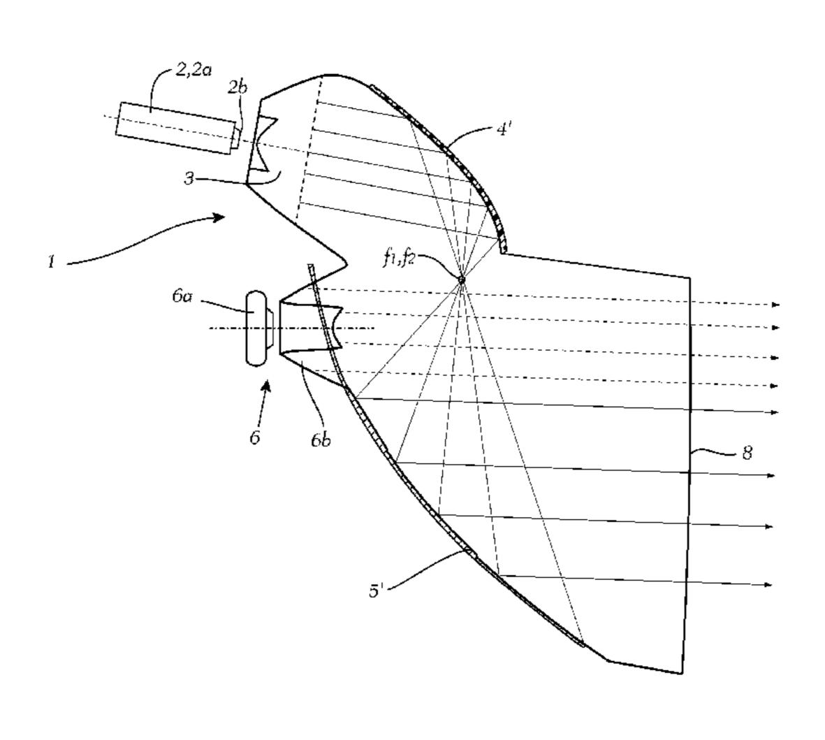
second light source arrangement (6) casts out an additional light output in the desired exit direction.
