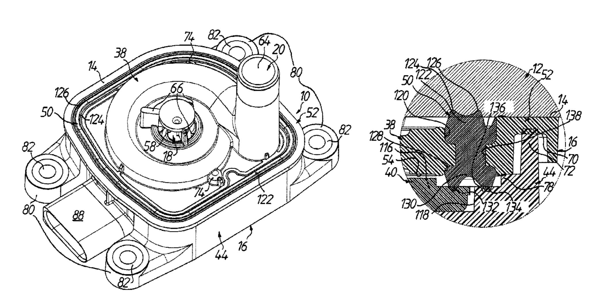
rotational axis, and a magnetic field sensor for detecting the position of the rotor. The housing includes a stator housing section which holds the stator, separates same from a liquid chamber in which the rotor is arranged, and extends into the rotor by a housing offset formed for receiving the magnetic field sensor.
