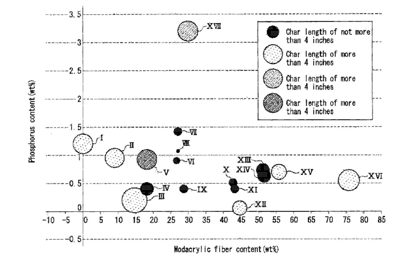
retardant fabric having a weight per unit area of not less than 160 g/m². The flame-retardant fabric can be produced by subjecting a fabric including a natural cellulose fiber and a modacrylic fiber containing an antimony compound to flame-retardant treatment with a phosphorus compound.
