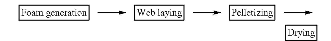
According to one preferred embodiment of the present invention, the web is compacted into pellets having an average size of 0.2 mm-40 mm (width) and 0.2 mm-40 mm (length), more preferably 0.2 mm-10 mm (width) and 0.5 mm-20 mm (length).
