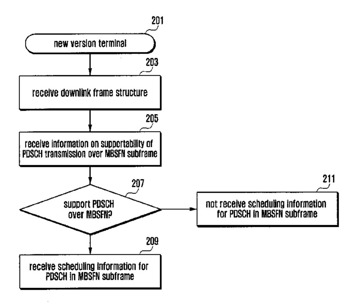
transmitting, to the terminal, the control information in the PDCCH and the data in the PDSCH in a second sub-frame of a non-MBSFN sub-frames, if the terminal is configured in the second transmission mode.
