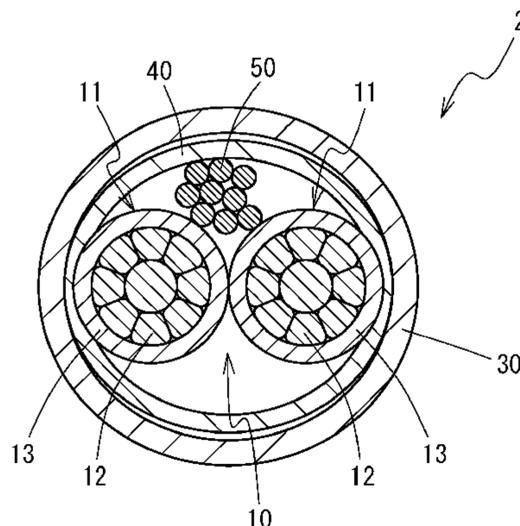
tensile strength of 400 MPa or higher, and an insulation coating that covers the conductor. The shielded communication cable 1 further contains a shield that is made of a conductive material and surrounds the twisted pair. The shielded communication cable has a characteristic impedance of  $100 \pm 10 \Omega$ .
