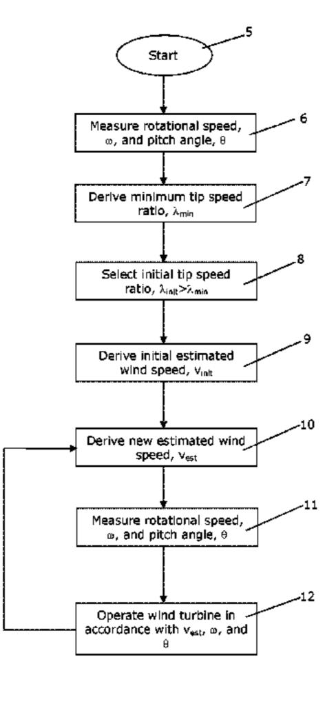
angle, a minimum tip speed ratio is derived as a limit or boundary point between a stable control region and an unstable control region.
