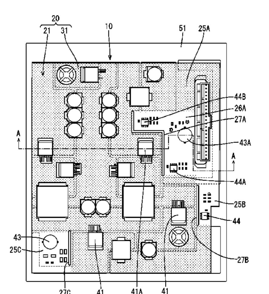
erate heat when current flows through it, and the other components are low heat resistant electrolytic capacitors and integrated circuits that are influenced by heat transferred from the semiconductor elements. Bus bar non-arrangement regions in which no bus bar is disposed are formed in the circuit structure, and the low heat resistant electrolytic capacitors and the integrated circuits are disposed in the bus bar non-arrangement regions.
