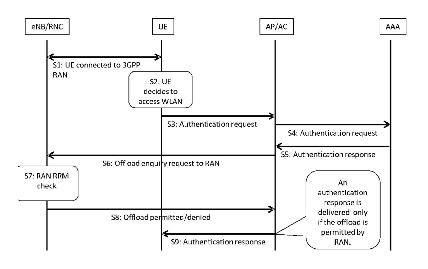
mitting a message indicating whether it is permitted to offload traffic to the access point of the wireless communication network.
