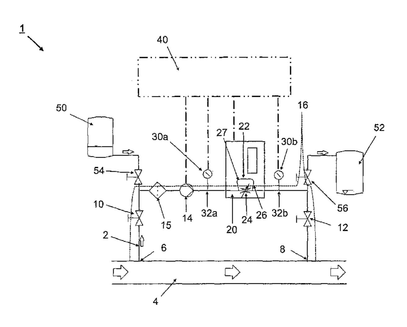
tains the density of the medium based on the volume flow, the volume flow dependent pressure drop and the at least one oscillatory characteristic of the oscillator.
