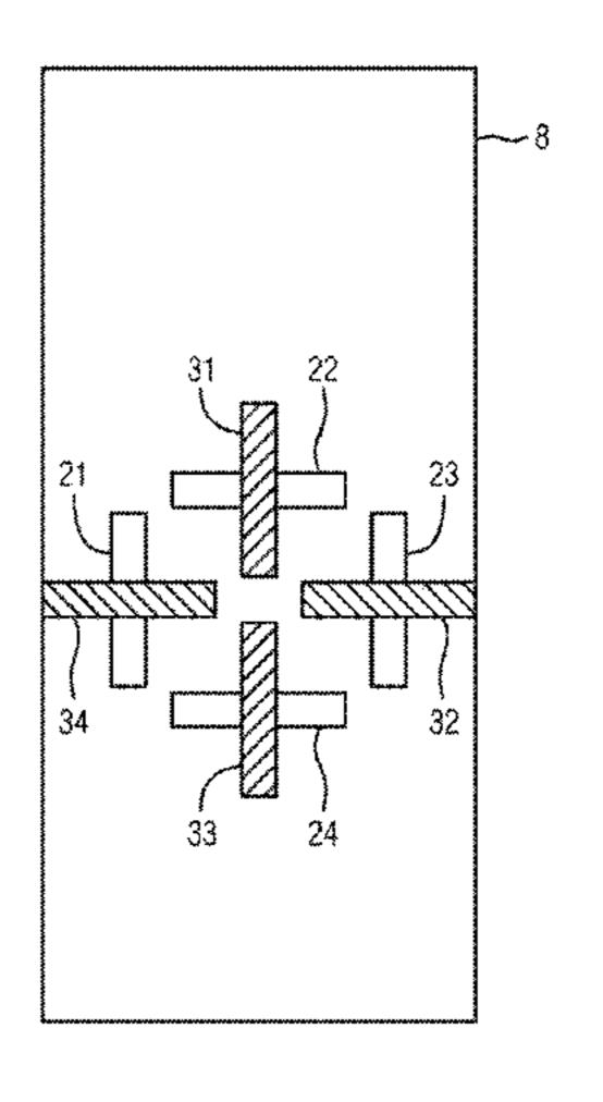
the charging station are movable at least vertically. The mutually complementary contacts are disposed in such a way that the contacts extend transversely to each other in a predefined charging position of the vehicle for establishing of the galvanic connection.
