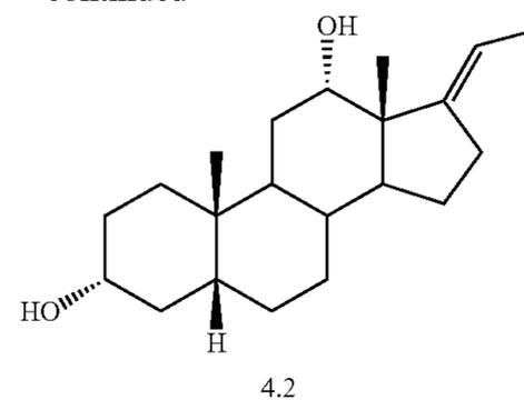
First the C<sub>17</sub> ketal and the C<sub>3</sub> silyl ether groups of Compound 2.2 are hydrolyzed. Then the Wittig reaction is performed to yield Compound 4.2. Conversion of Compound 4.2 to Compound 5.1 is carried out via an ene reaction. Subsequent catalytic reduction of Compound 5.1 and hydrolysis of the ester yields DCA (Scheme 5).
