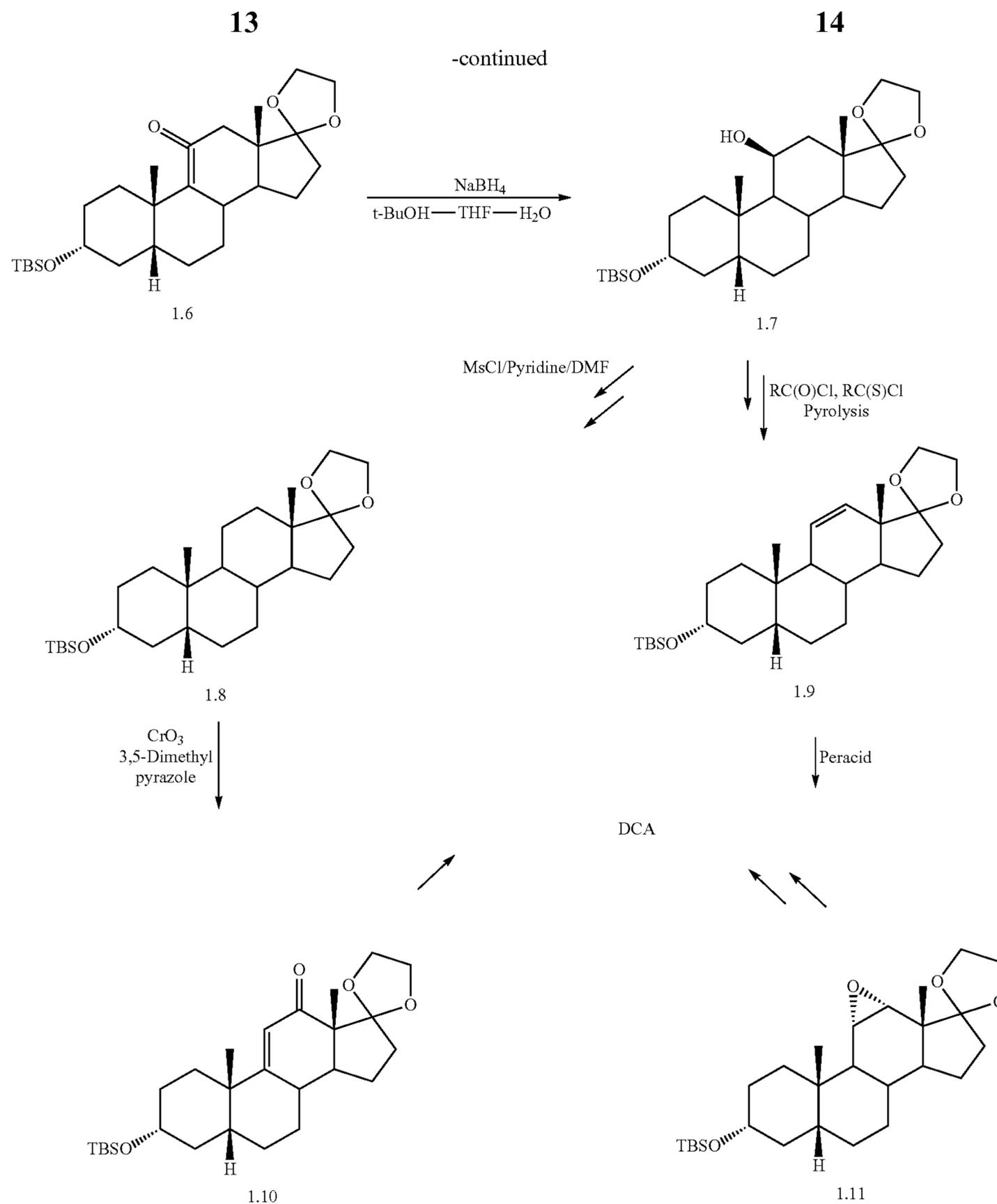
Allylic oxidation of Compound 1.8 (via treatment with CrO<sub>3</sub> and 3,5 dimethyl pyrazole) yields the enone-containing Compound 1.10. Peracid oxidation of Compound 1.9 proceeds stereoselectively from the alpha-face of the steroid to yield the C<sub>11-12</sub> epoxide Compound 1.11 (see Scheme 1A above). These chemical transformations yield the two key precursors of the C<sub>12</sub> hydroxyl group functionality, namely, Compound 1.10 and Compound 2.1 (Schemes 1A and 2).
