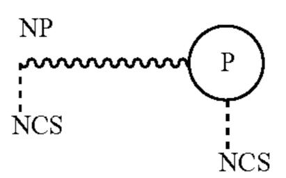
wherein the protonated form of the surfactant comprises a non-polar moiety (NP) and a polar moiety (P), and wherein at least one isothiocyanate functional group (NCS) is associated with the polar and/or non-polar moiety.
