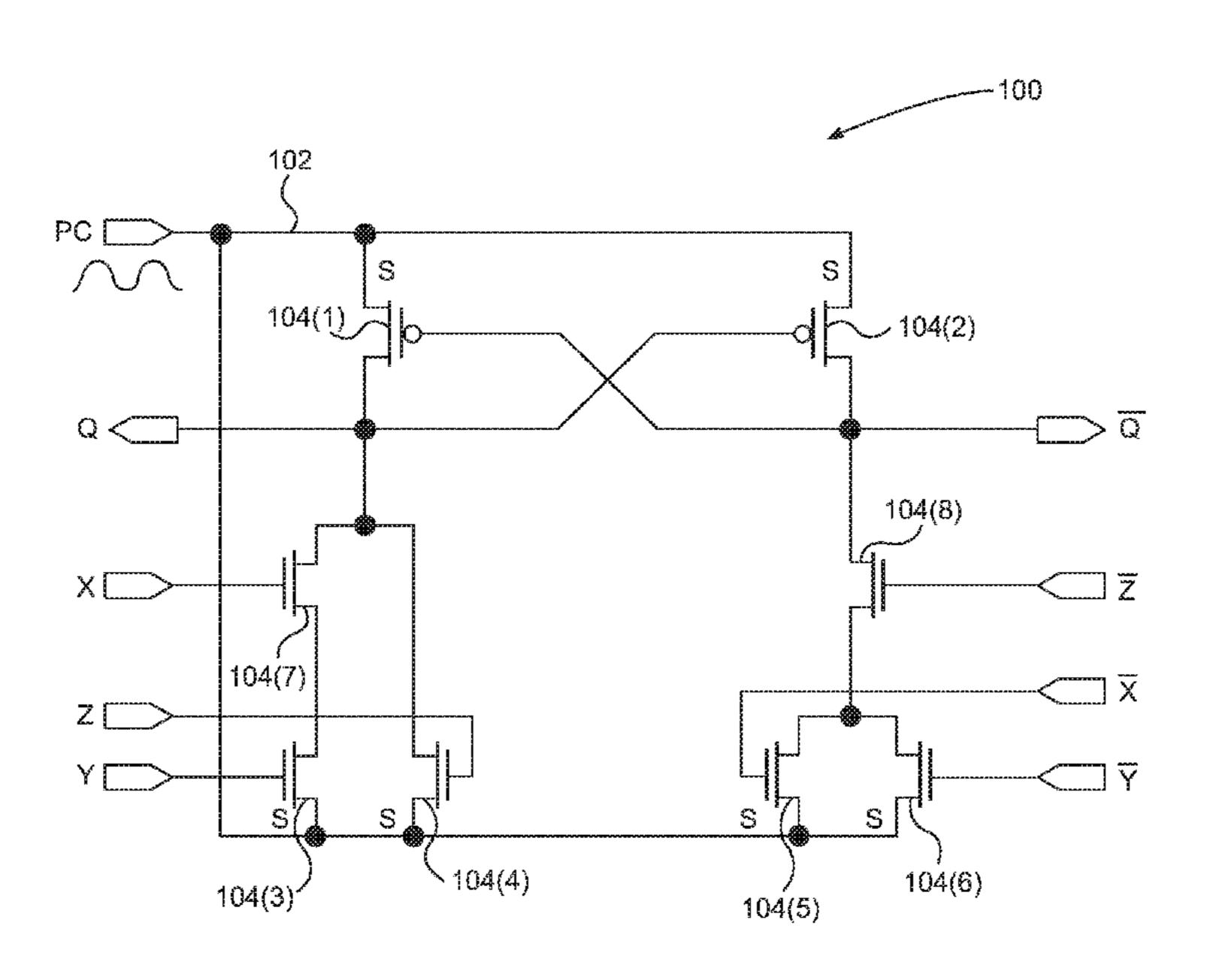
logic circuit. The AC power signal is provided to the power rail to provide power to the adiabatic logic circuit. Wirelessly charging the adiabatic logic circuit consumes less power than conventional non-wireless charging circuitry.
