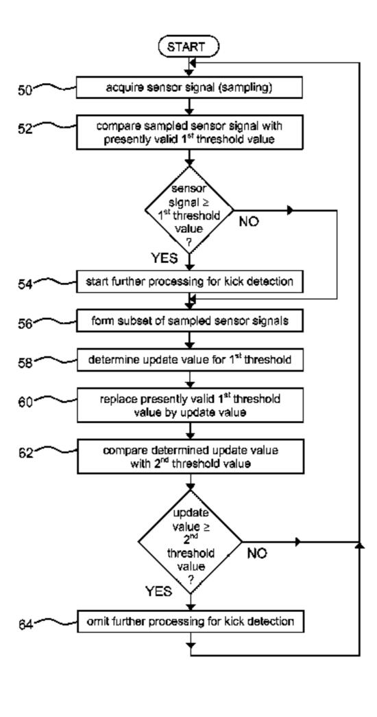
than or equal to the presently valid first threshold value, forming a subset out of the sampled sensor signals, determining an update value for the first threshold value, and replacing the presently valid first threshold value by the update value.
