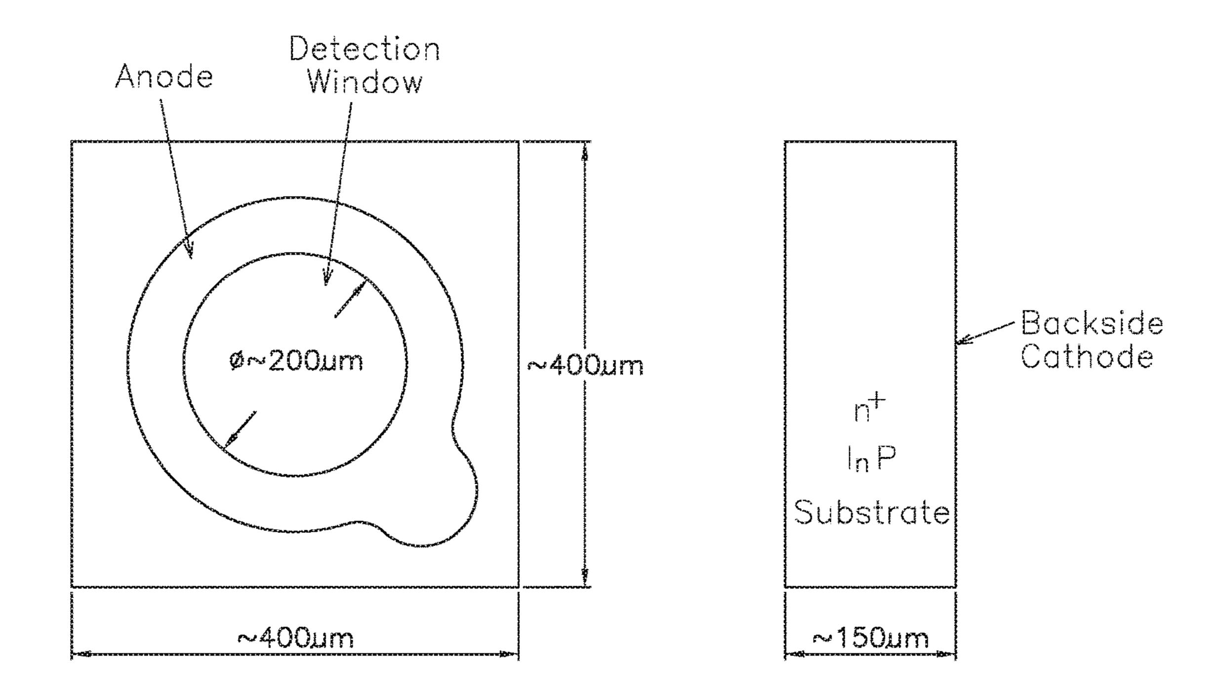
In Ga As Monitor Pin Photodiode Fig. 5 Prior Art
