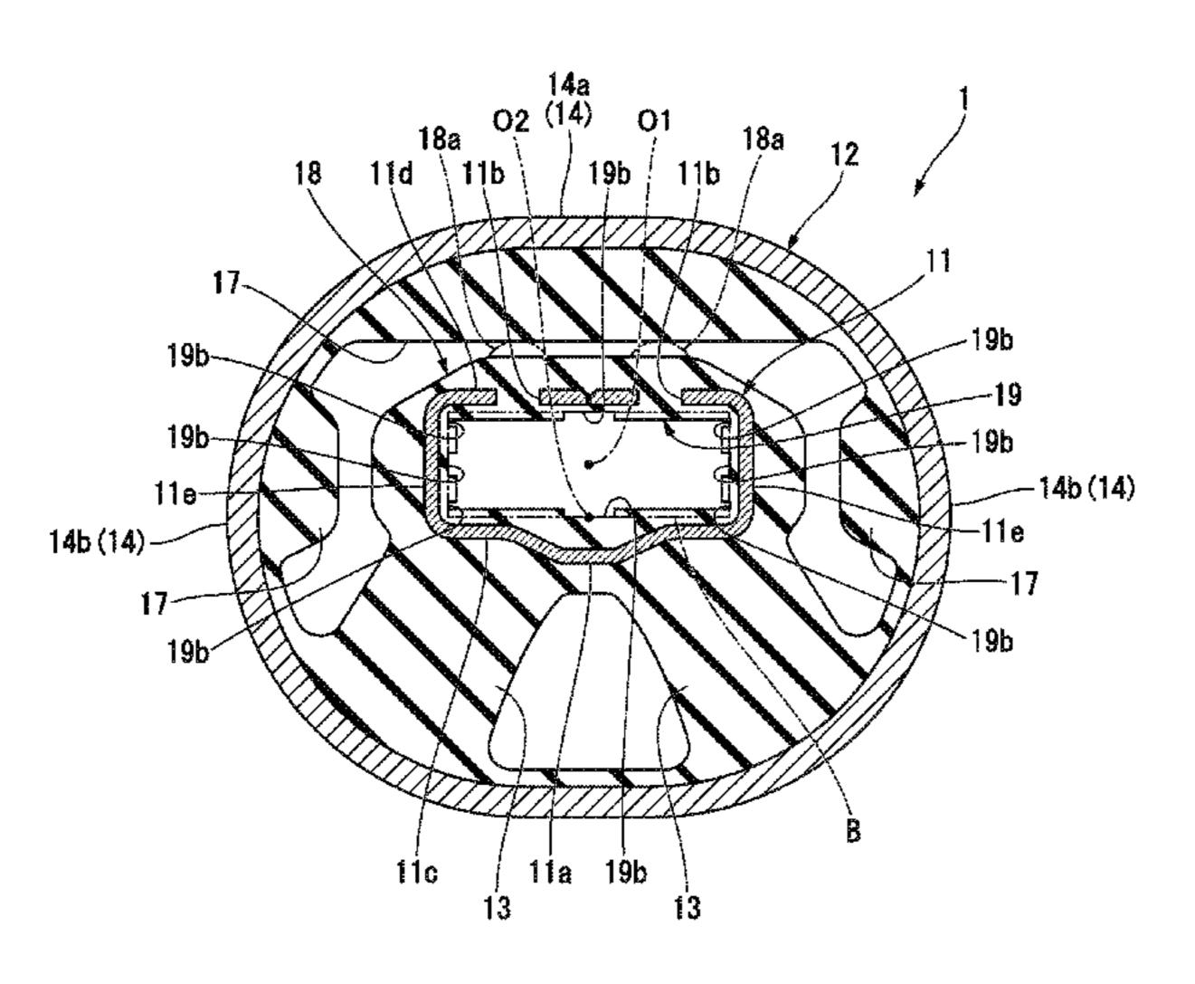
protrudes to an outer circumferential surface side of the first attachment member through the penetration hole.
