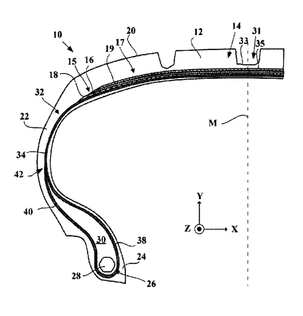
least one layer of a thermoplastic polymer composition. The ratio R1=ODO/E of the mean minimum thickness ODO of elastomer present on the back of the sheath to the mean thickness E of the reinforced product (21) is less than or equal to 0.17, the mean minimum thickness of elastomer ODO and mean thickness E of the reinforced product (21) being measured in a direction substantially perpendicular to the main direction (X1).
