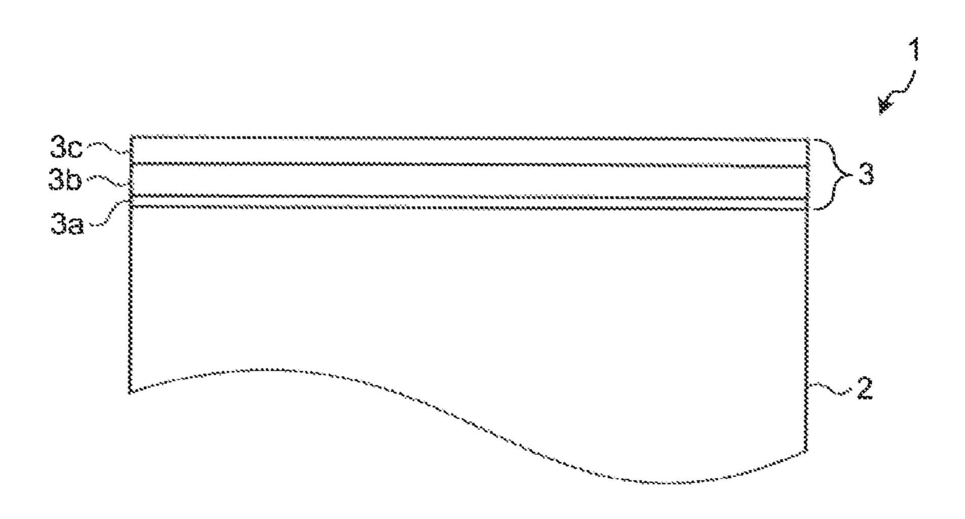
containing terephthalic acid as a polycarboxylic acid component and 1,4-butanediol as a polyol component both of which are 90 mol % or more of the respective components, has a total thickness of 3 to 25  $\mu$ m, and has a ratio (I011/I100) of peak intensity (I011) observed in the range of  $2\theta$ =15.5 degrees to 17.0 degrees to peak intensity (I100) observed in the range of  $2\theta$ =22.5 degrees to 24.0 degrees in X-ray diffraction in the range of 0.2 to 5.0.
