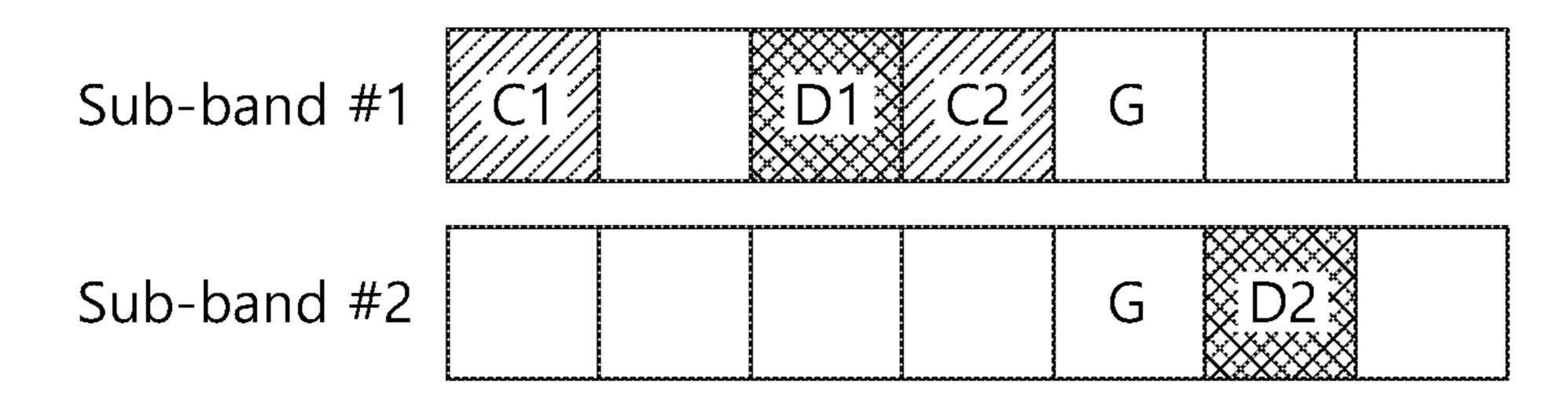
: subframe on which MPDCCH transmission is completed
