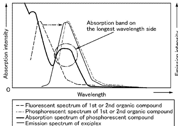
first phosphorescent compound, a first organic compound having an electron-transport property, and a second organic compound having a hole-transport property and is provided on the anode side, and a second light-emitting layer, which contains at least a second phosphorescent compound and the first organic compound having an electron-transport property. A combination of the first organic compound and the second organic compound forms an exciplex.
