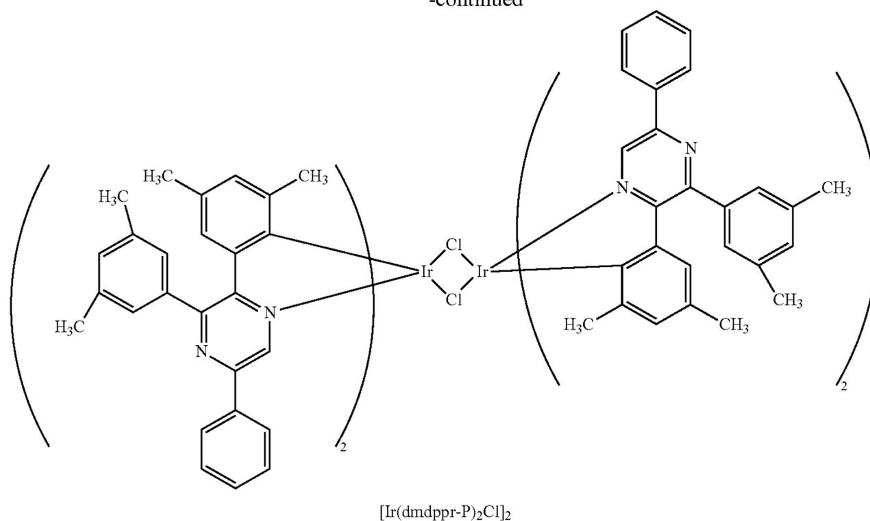
Step 4: Synthesis of Bis{4,6-dimethyl-2-[3-(3,5-dimethylphenyl)-5-phenyl-2-pyrazinyl-κN]phenyl-κC}(2,6-dimethyl-3,5-heptanedionato-κ<sup>2</sup>O,O') iridium(III) (abbreviation: [Ir(dmdppr-P)<sub>2</sub>(dibm)])
