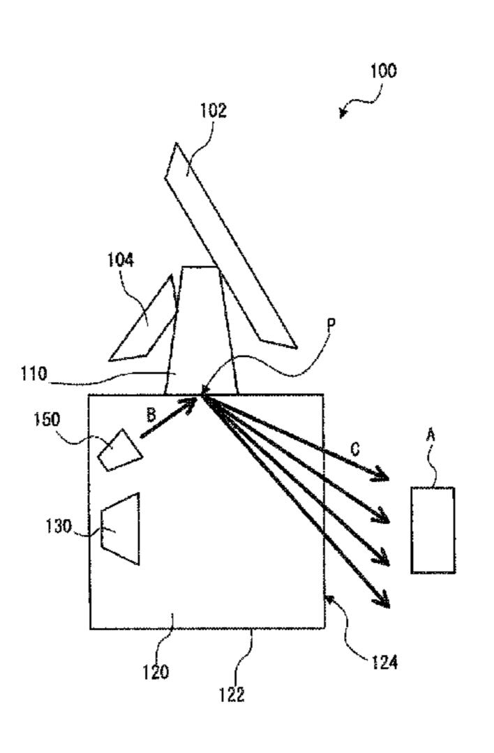
the brightness of the environmental light measured by the brightness measurement unit (2). The image pickup unit (6) shoots the commodity irradiated with the light by the irradiation unit (4) and thereby generates an image thereof. The recognition process unit (8) performs a process for recognizing the commodity based on the image generated by the shooting performed by the image-pickup unit (6).
