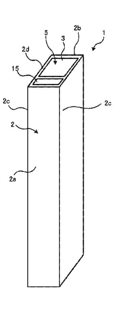
entrance plane and the light exit plane; and a wavelength conversion layer having quantum dots that is placed in the receiving space. The distance between the light entrance plane and the wavelength conversion layer is longer than the distance between the light exit plane and the wavelength conversion layer.
