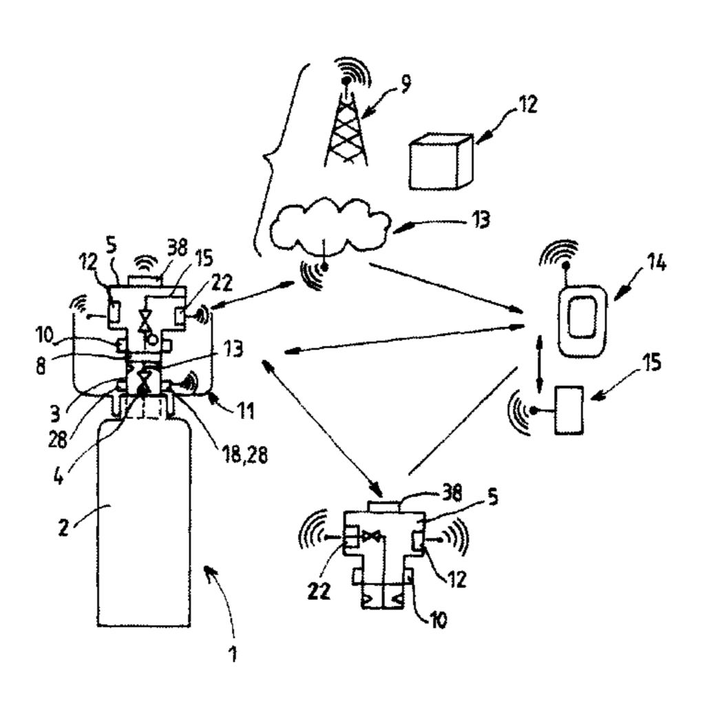
first tap and a second tap connected detachably to the first tap, and the electronic communication apparatus being situated either on the cylinder, on the cap, on the first tap, or on the second tap.
