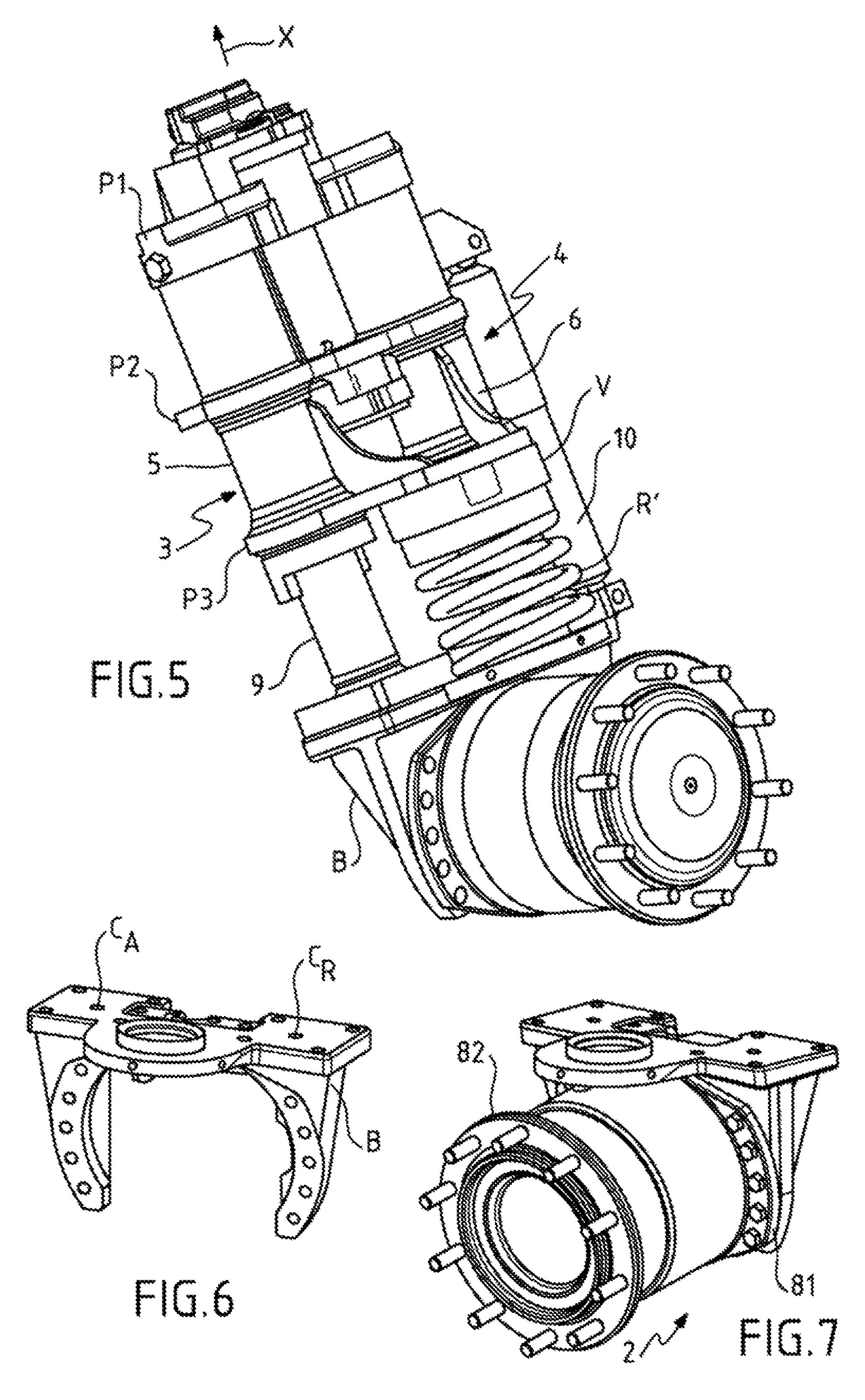
METHOD OF SUPPLYING A HYDRAULIC MOTOR FOR A DRIVE WHEEL WITH HYDRAULIC FLUID, ASSOCIATED CYLINDER-TYPE SUSPENSION SYSTEM AND VEHICLE EQUIPPED THEREWITH
