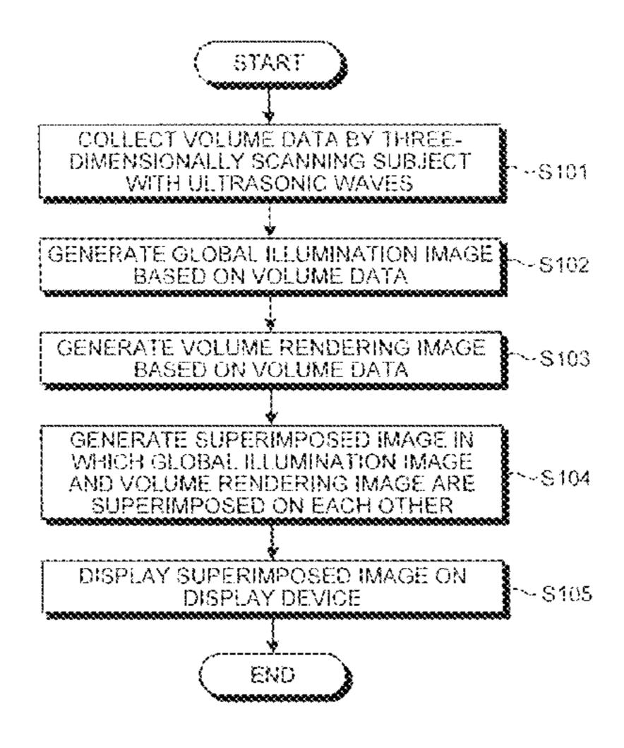
second rendering image are superimposed on each other. The display control unit causes a display device to display the superimposed image. The superimposition processing unit adjusts a superimposition ratio of the first and second rendering images in the superimposed image.
