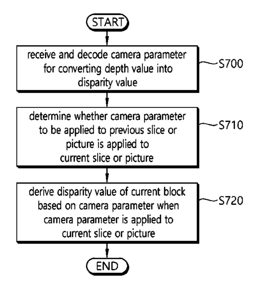
parameter applies to a current slice or picture, deriving a disparity value of a current block on the basis of the camera parameter. According to the present invention, slices or pictures of a certain interval may share the same camera parameter, the transmission of overlapping information may be prevented, and coding efficiency may be improved.
