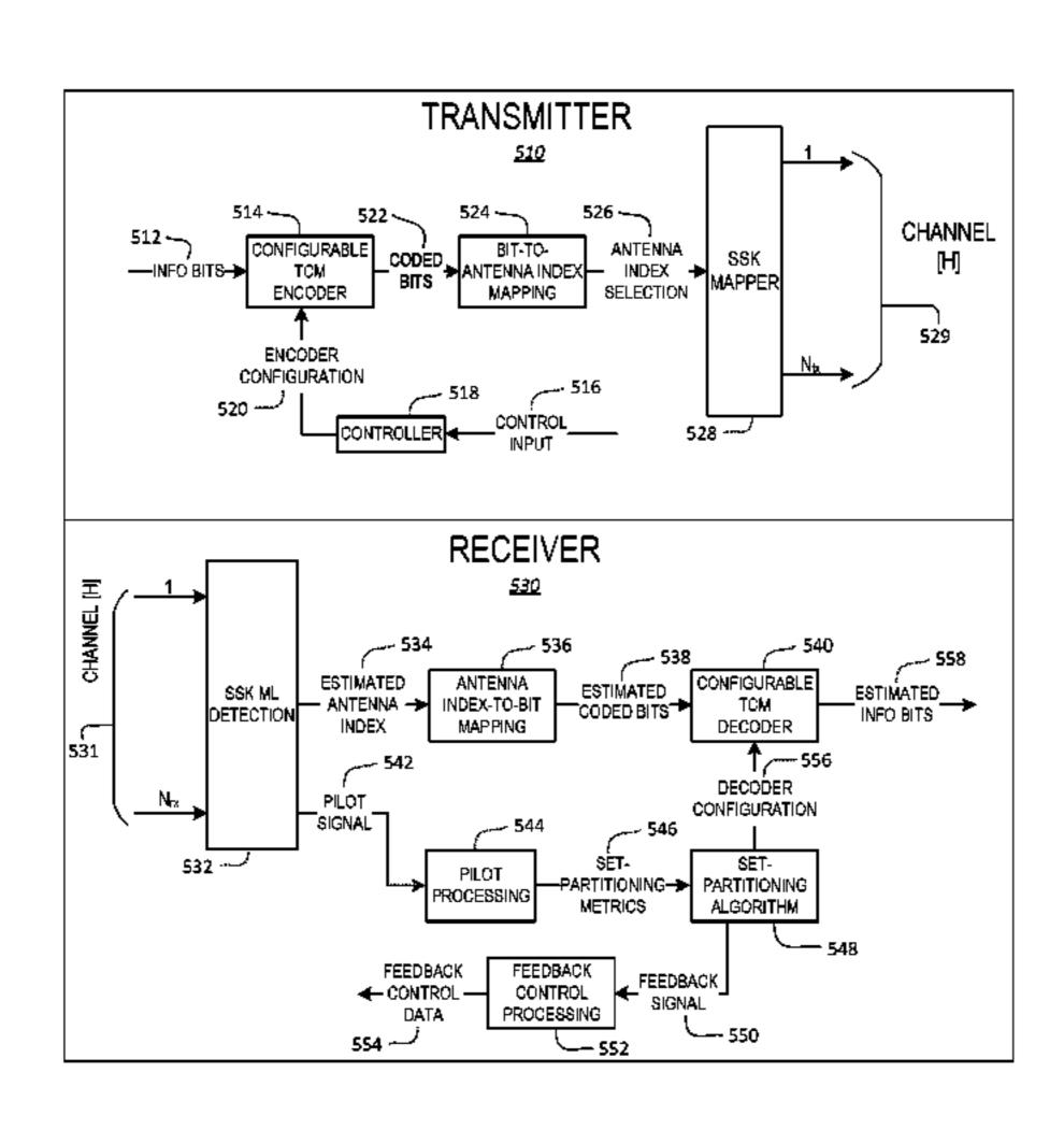
Coded Modulation (TCM) decoder based on the determined set-partition.
