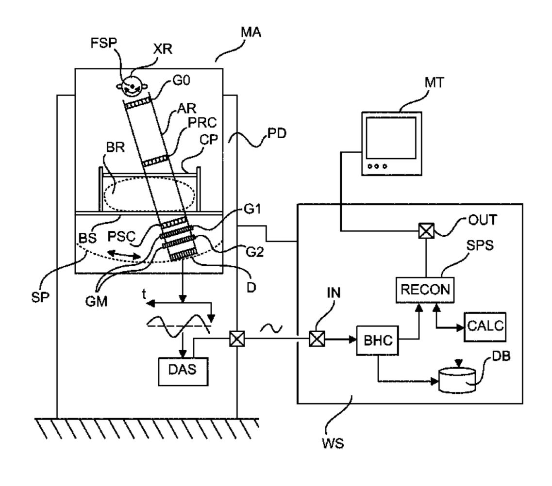
position or geometric ray of an imaging region of the apparatus (MA). In one embodiment, a phantom body (PB) is used to acquire calibration data on which the beam hardening processing is based.
