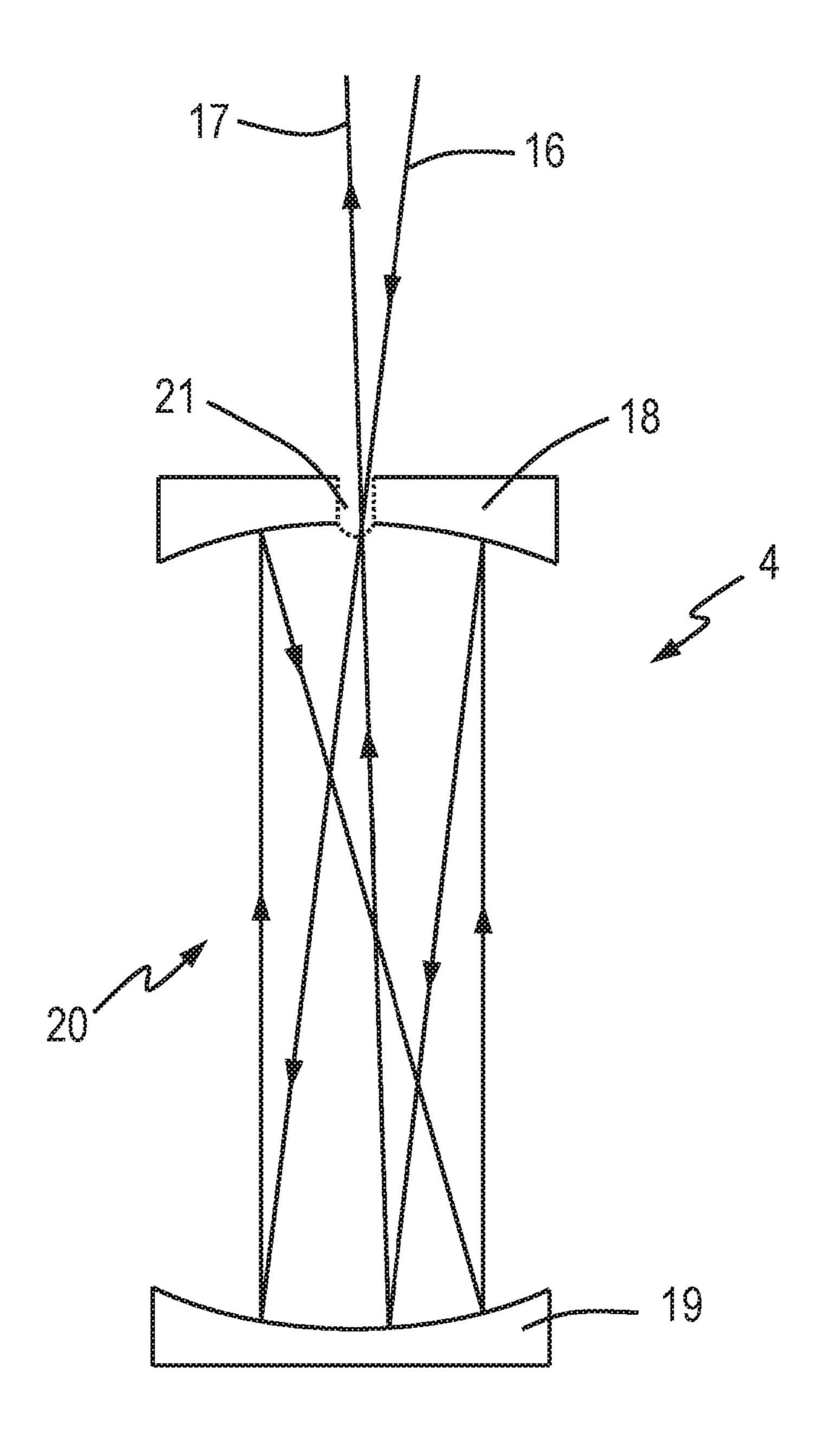
Provide a Multi-pass Absorption Cell with a Vapour Sample Taken From around the Perimeter of One or More Casks
