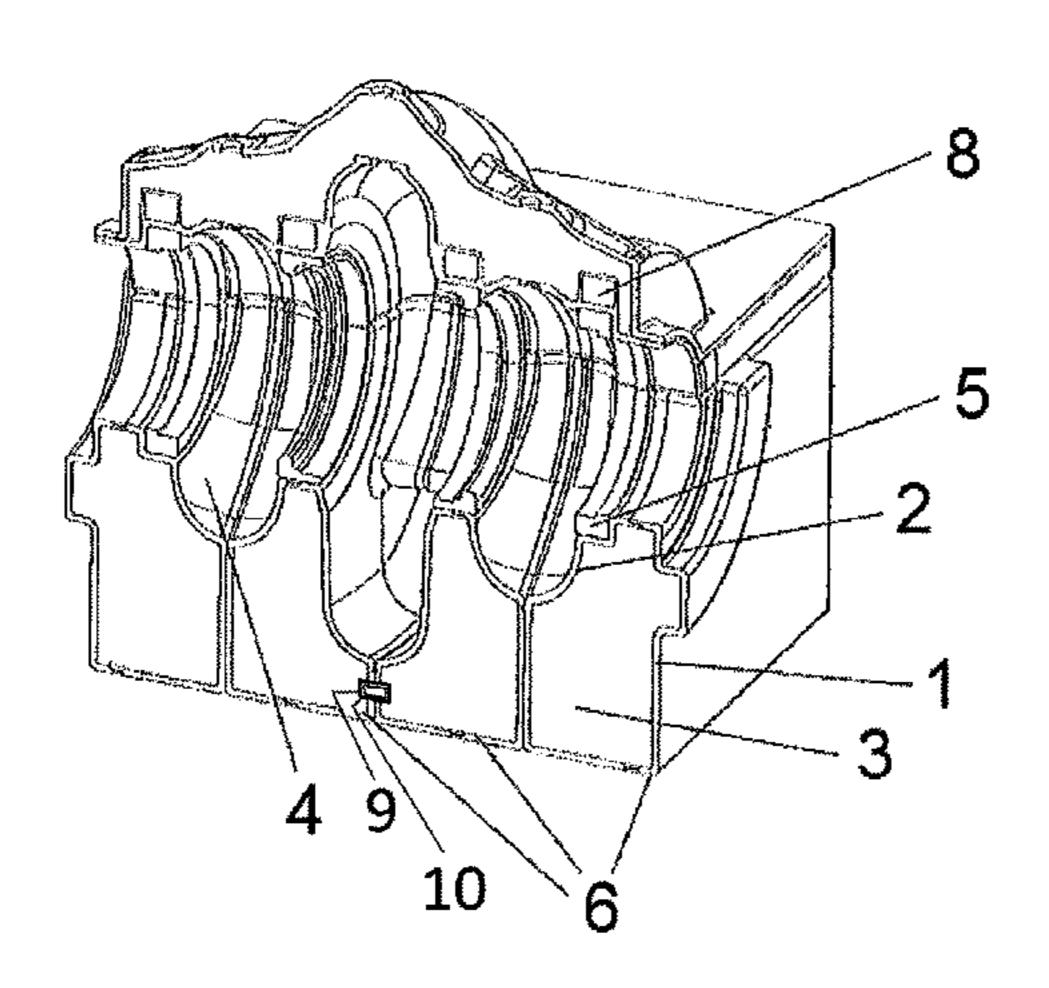
dimensionally stable, with a space between the first casing and the second casing. A filler material such as a selfexpanding foam may be provided in the space. The pump casings may be standardized components, and multiple casings may be assembled to form pump housings to suit a particular application.
