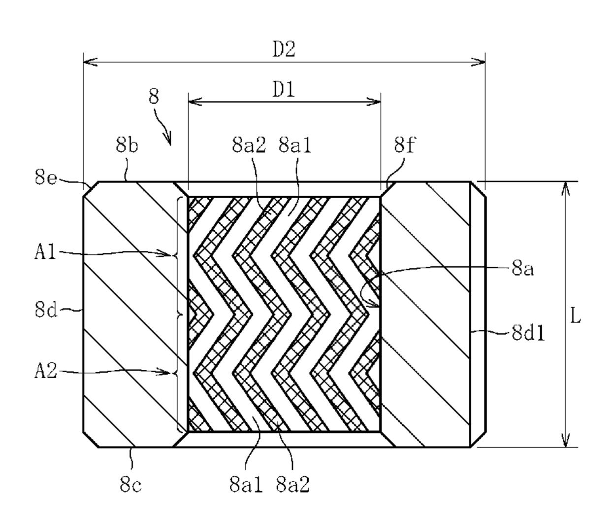
sintered metal bearing is set to 6 mm or less, and a density ratio of the sintered metal bearing is set to 80% or more and 95% or less.
