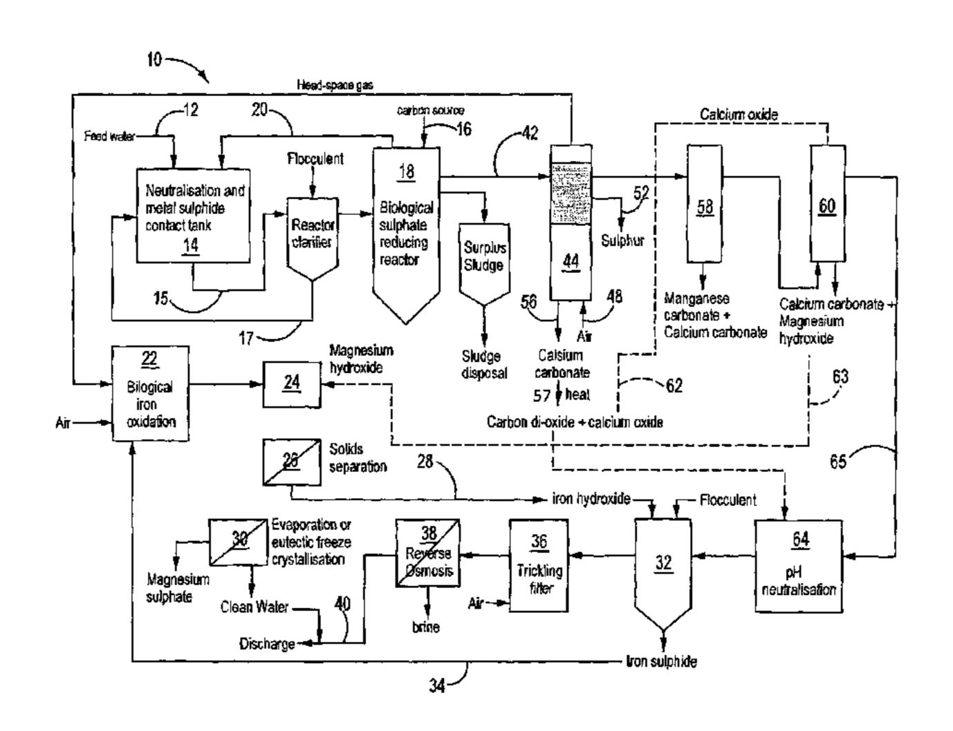
bed reactor at a sufficient rate to effect abrasion to remove elemental sulphur from the floating media, harvesting the sulphur from a top portion of the reactor, recycling hydroxyl ions internally in solution in to enhance calcium carbonate precipitation by further increasing the pH.
