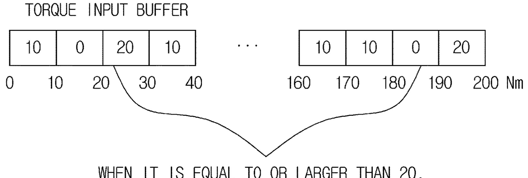
WHEN IT IS EQUAL TO OR LARGER THAN 20, SET THAT ALL TORQUE SAMPLES IN CORRESPONDING SECTION ARE OBTAINED
