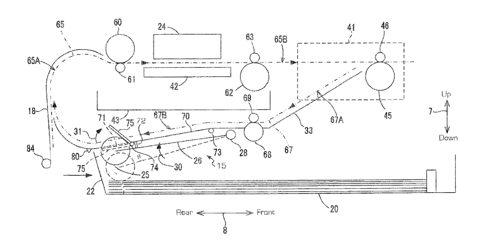
from the sheet holding surface. A return guide, disposed between the recording unit and the sheet feeder, defines a second conveying path to guide the sheet having an image recorded on one side thereof back to the feed guide. The return guide has a first opening configured to accommodate the roller of the sheet feeder when the roller is in the second roller position.
