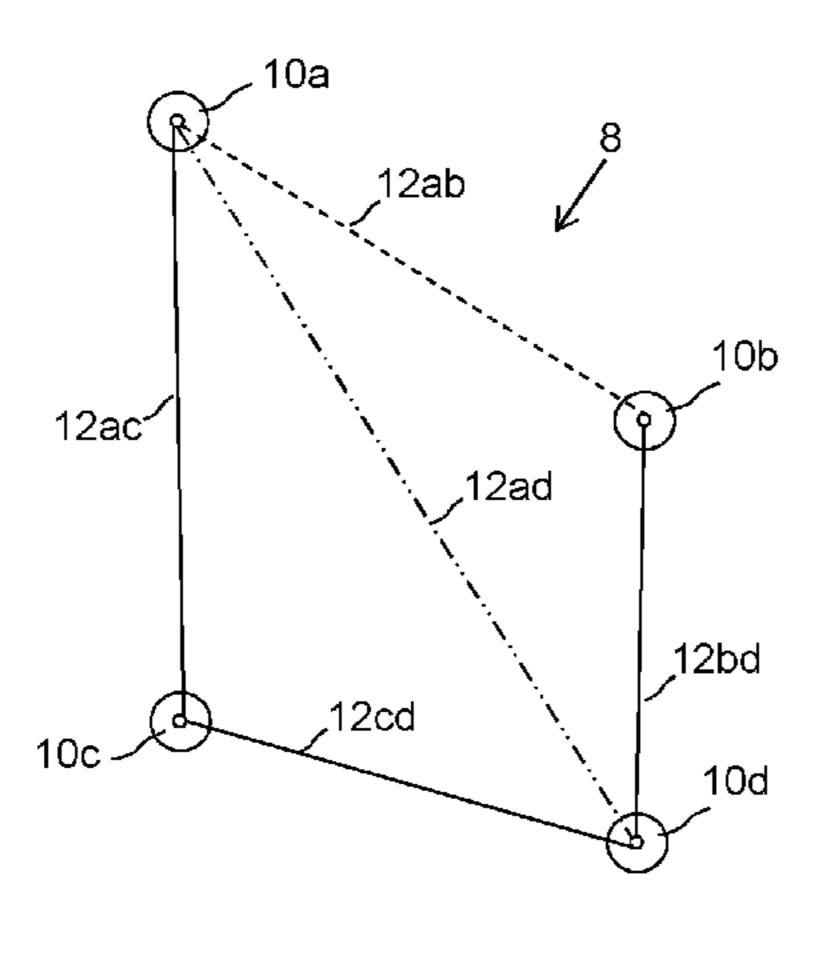
video) not supported by the first link class. Data may then be routed across the network (8) while ensuring that only data of types consistent with the link classes assigned to respective links (12ab, 12ac, 12bd, etc) are transmitted via those links.
