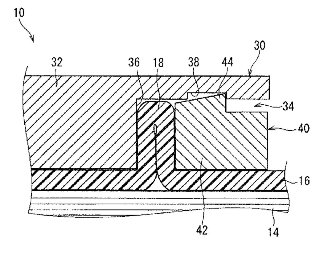
contact with the step, and a retainer to be locked to the connector housing with the bulge pressed toward the step.
