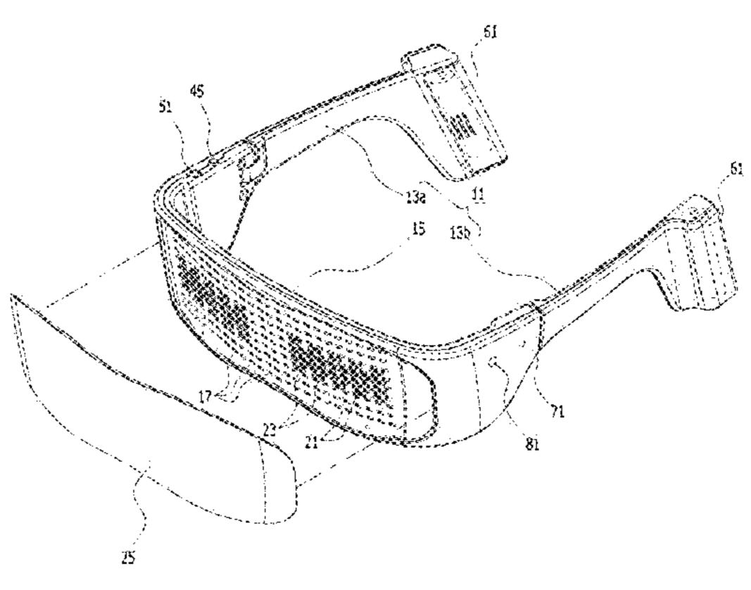
frame, for controlling the operation of the light-emitting diodes so that the first pattern data or the second pattern data are displayed via the light-emitting diodes.
