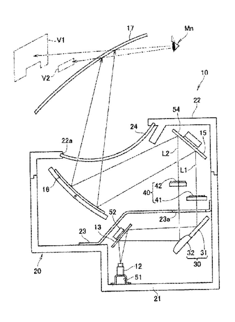
device reaches the first screen is different from the length of a second optical path in which the light emitted from the light-emitting device reaches the second screen.
