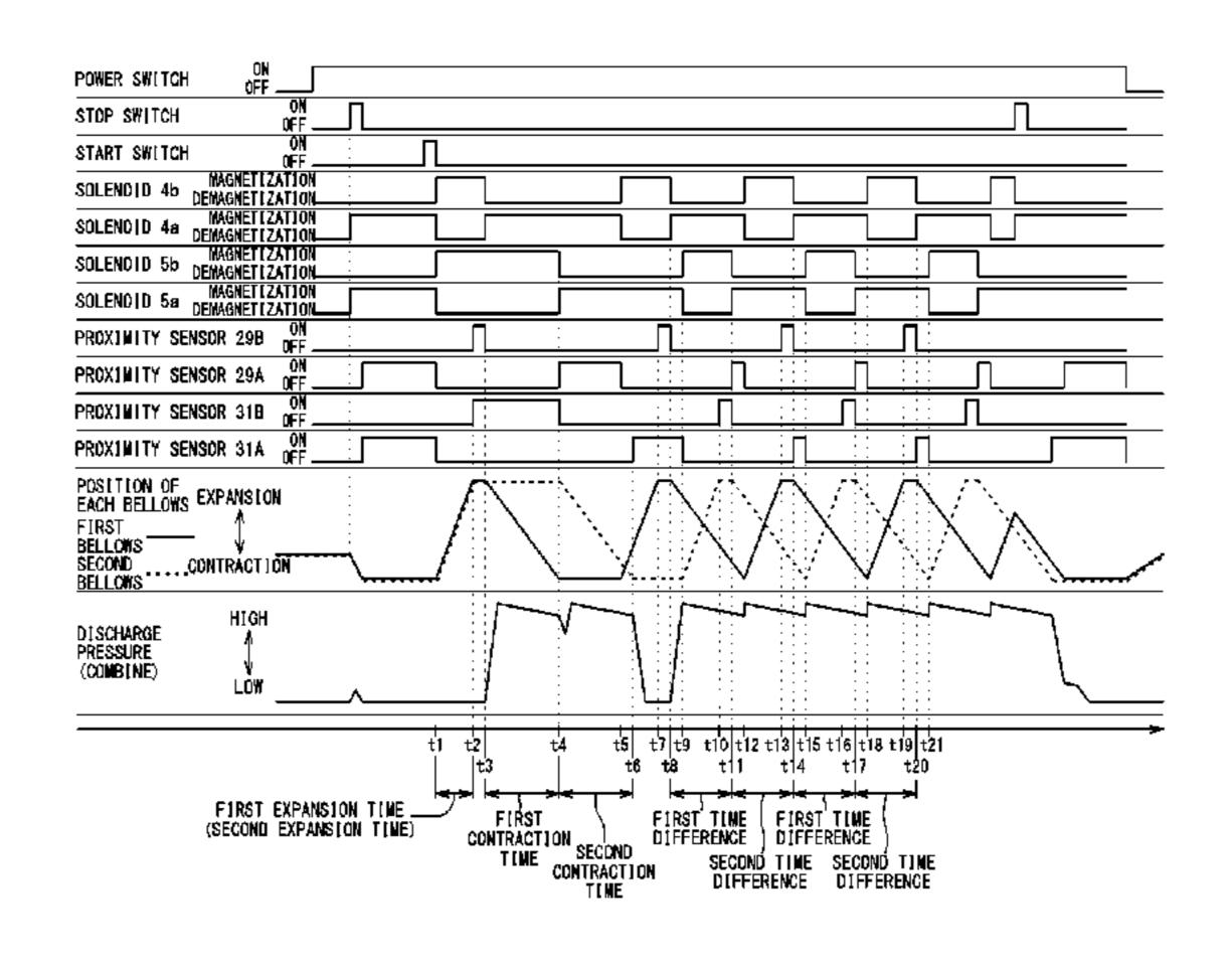
of detection signals of the first and second detection devices such that, before one bellows comes into a most contracted state, the other bellows is caused to contract from a most expanded state.
