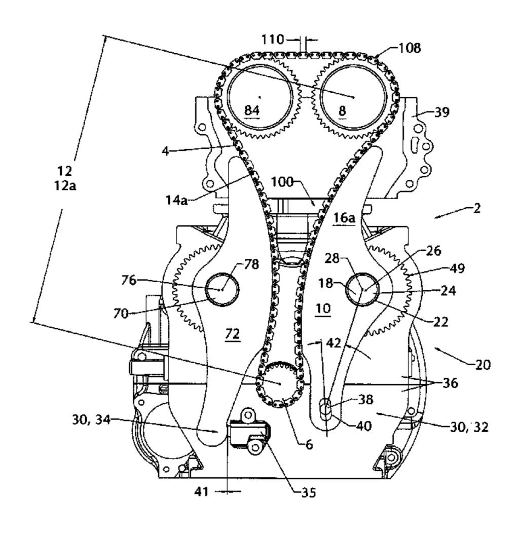
drive pulley mounted on the crankshaft and the driven pulley mounted on the camshaft. The system provides slackless operation of the endless band at two or more compression ratio values.
